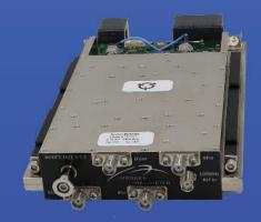
We developed a state of the art NUDC2-18/1.3-2.3 Wideband Microwave Transceiver in a low-SWaP 3U module. The NUDC2-18/1.3-2.3 is a dual conversion Transceiver providing 2-18 GHz operation in a versatile OpenVPX platform. The NUDC2-18/1.3-2.3 includes internal LOs which provide an instantaneous IF bandwidth of 1 GHz and exceptional Noise Figure.
